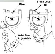
**GENERAL INSTRUCTIONS** - The removable Risers are to accommodate different sizes of cable. It is through the use of Risers of different height that one instrument is able to measure tensions of various cable sizes (depending on the model). **The correct Riser must be used for the cable size under test; otherwise false readings or damage to the instrument will result.** Consult the Calibration Card (included) for tension range, cable size and proper riser.
