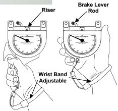
**GENERAL INSTRUCTIONS** - The removable Risers are to accommodate different sizes of cable. It is through the use of Risers of different height that one instrument is able to measure tensions of various cable sizes (depending on the model). The correct Riser must be used for the cable size under test; otherwise, false readings or damage to the instrument will result. Consult the Calibration Card (included) for tension range, cable size and proper riser.
